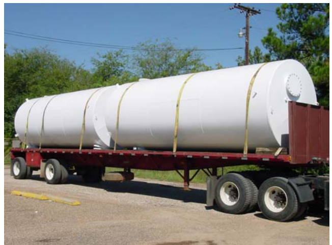
8,000 gallon API 650 tanks
