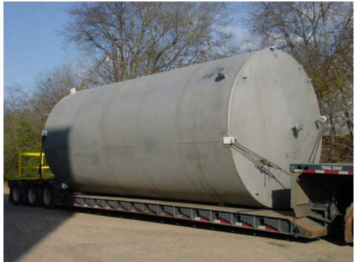
20,000 gallon stainless steel water tank.
