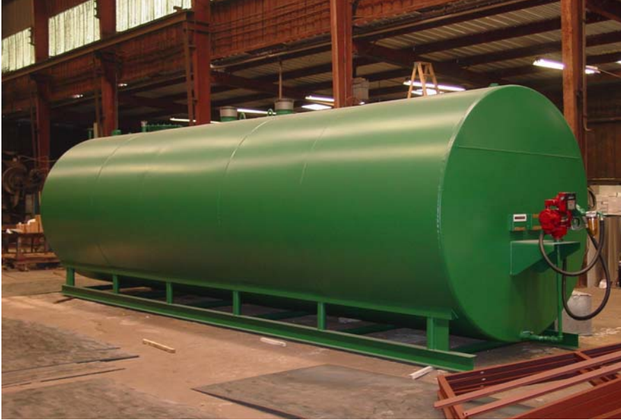
8,000 gallon UL142 double wall skid tank with dispensing system.
