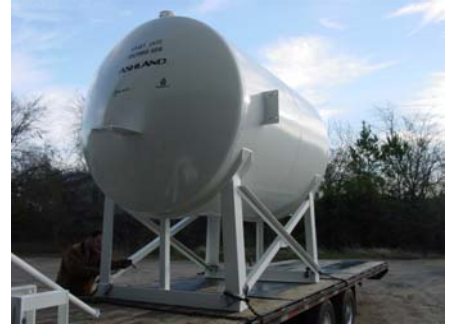
3,000 gallon chemical tank on 3' welded stand assembly.
