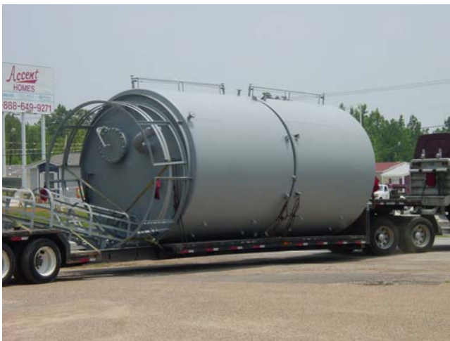
Two 5,000 gallon UL142 tanks with OSHA guardrails and ladders and sight gages.
